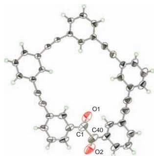
Figure 1. ORTEP view of 4 . Selected bond lengths and angles: C1–O1 = 1.226(3) Å, C40–O2 = 1.229 Å, C1–C40 = 1.524 Å, O1–C1–C40 = 116.9(3)°, and O2–C40–C1 = 119.5°.
